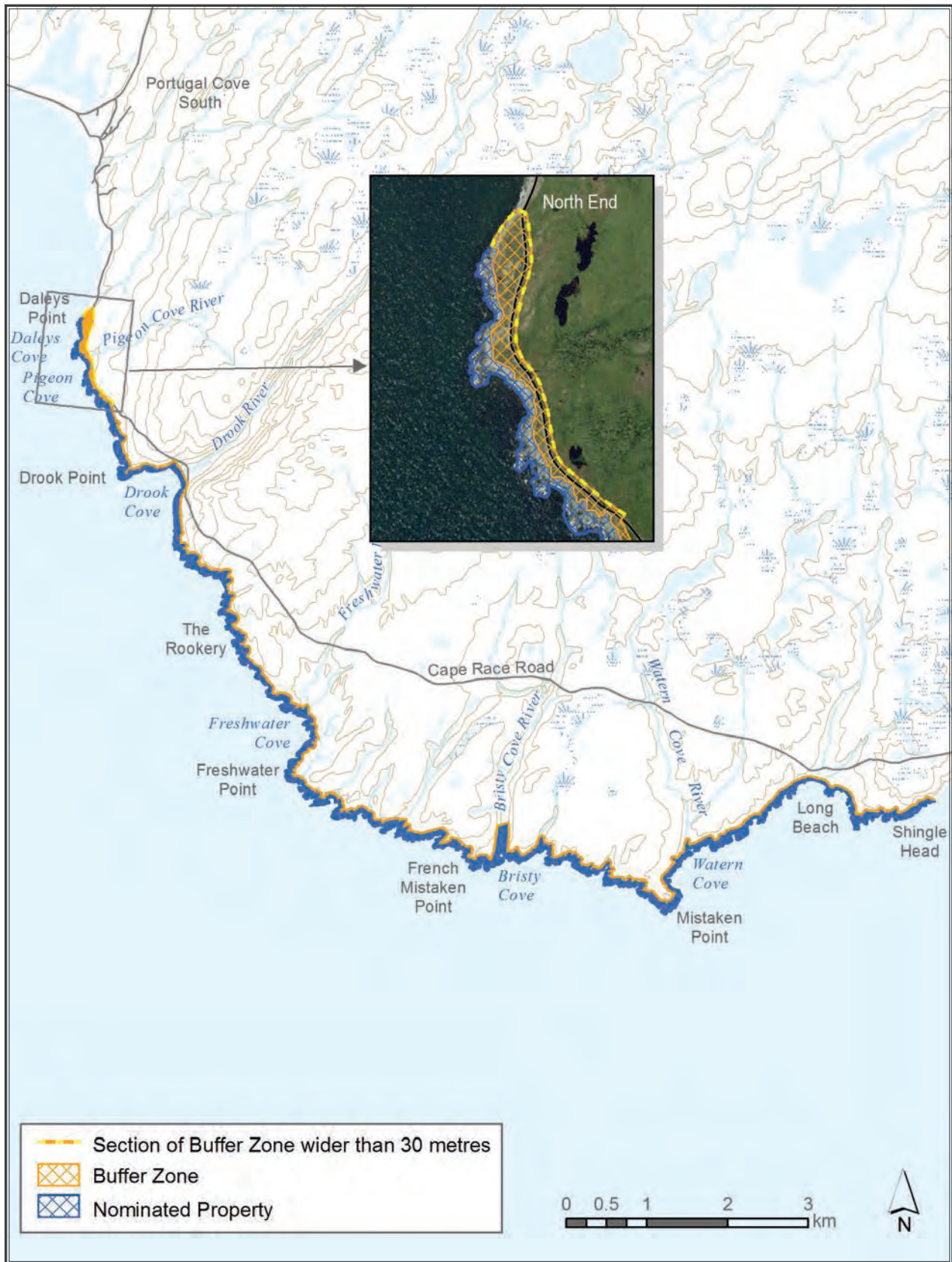
Figure 1.7. The majority of the buffer zone extends 30 metres inland from the landward boundary of the property; the buffer zone is wider in one location due to higher rates of erosion (inset).
